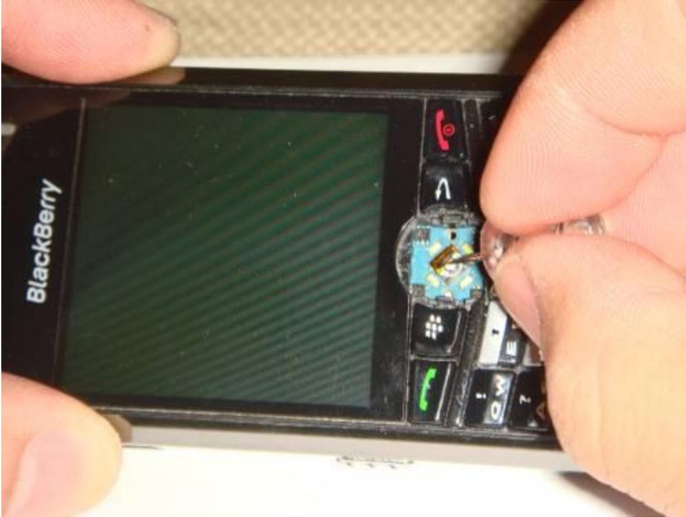
The next step is to take your q-tip (dipped mine in a little bit of rubbing alcohol, squeezing any excess out) and clean both the contact that is in the BB as well as that piece that you peeled off.
